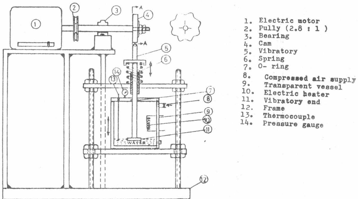
Fig. 1. Diagrammatic arrangement of experimental vibratory apparatus.
