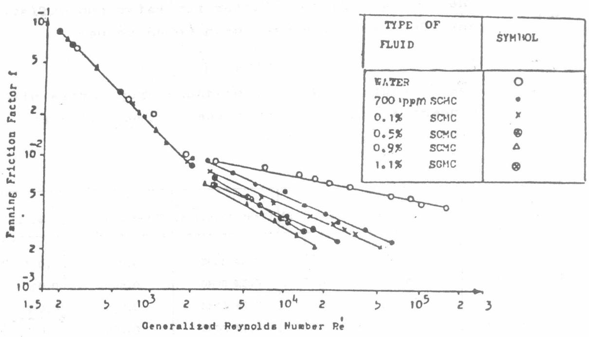
Fig.(4), Fanning Friction Factor for 17.5 mm pipe.
