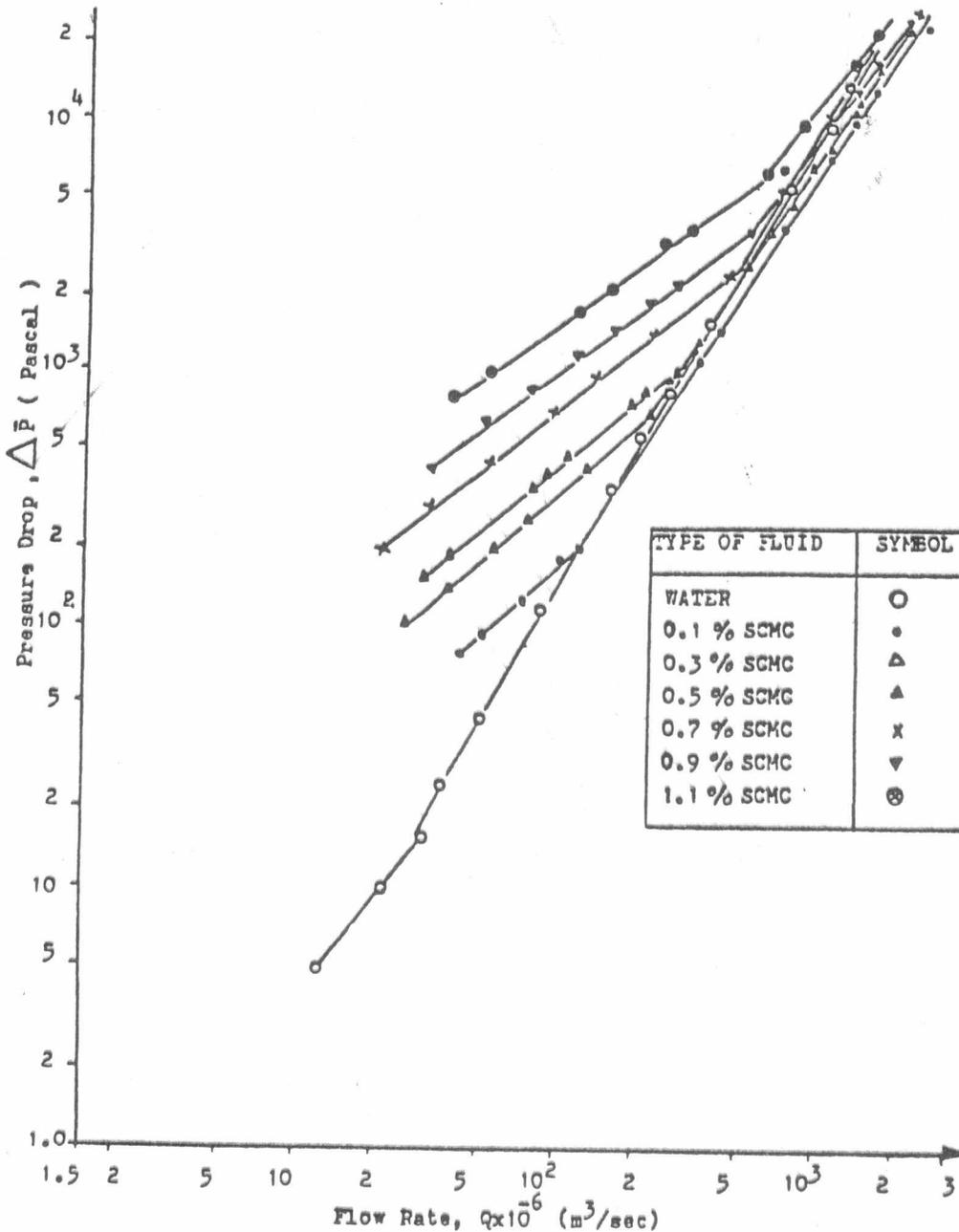
Fig.(2), Pressure drop in 17.5 mm smooth pipe.
