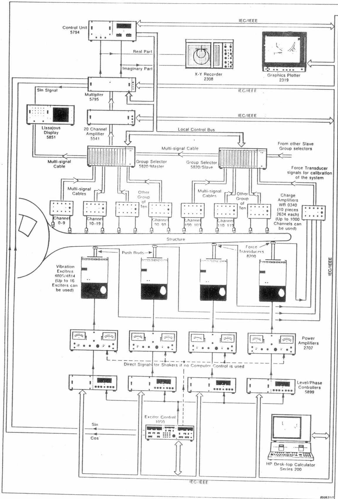
Fig.4 Instrumentation set-up for testing of large structures using multiple shakers
