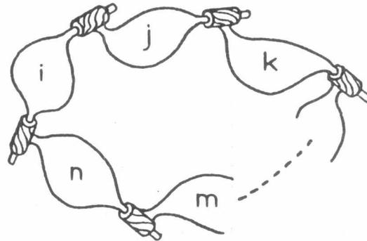
Fig. 4 Single closed loop of rigid bodies.
