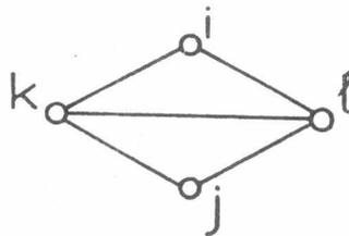
Fig. 1 Coupling graph of a kinematic chain with cross-jointing.
