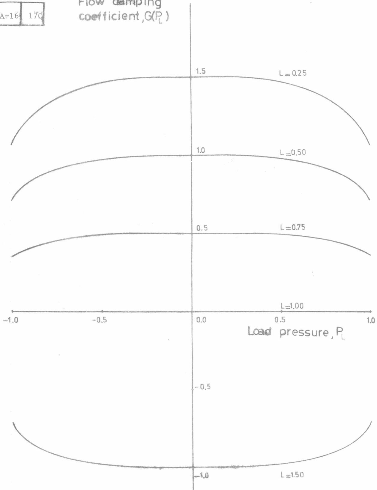
Fig.2 Dimensionless flow damping coefficient in underlap region
