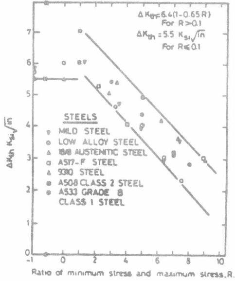
Fig. 5. Effect of stress ratio on  $\Delta K_{th}$ .
