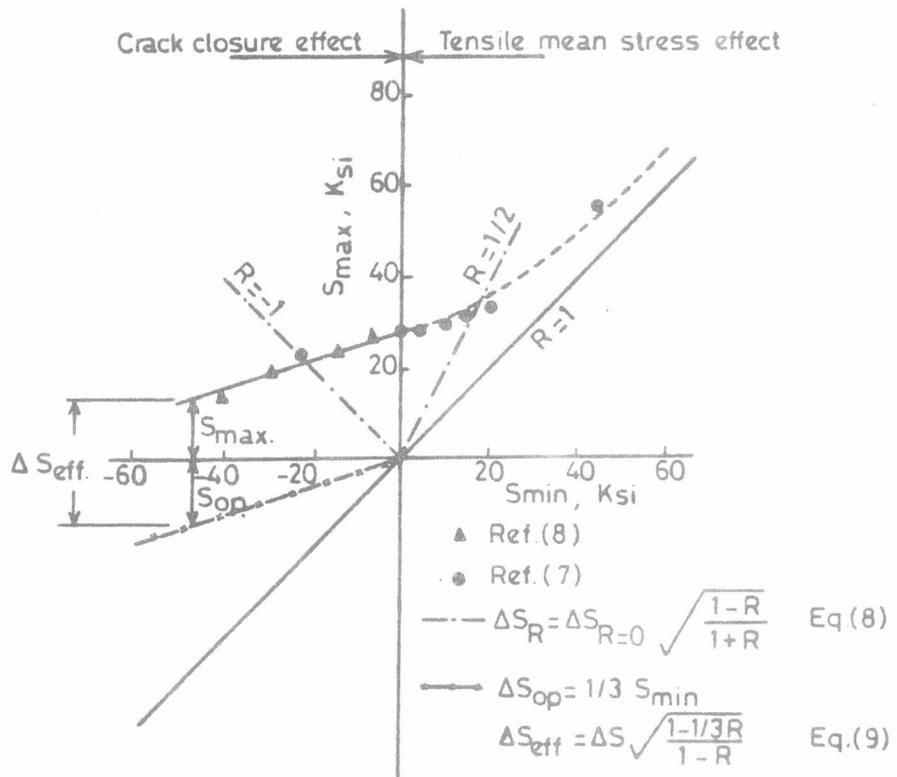
Fig.9 Relation between  $\Delta S_{eff}$  and mean stress.
