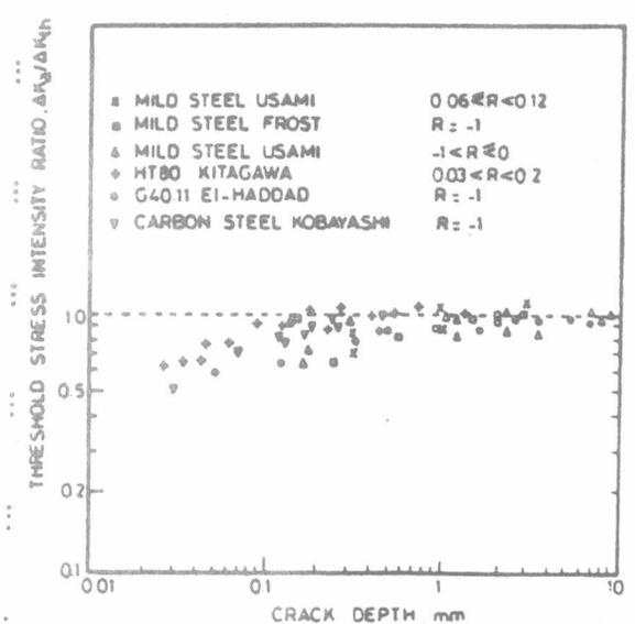
Fig.2. Relationship between crack depth and threshold stress intensity ratio  $\Delta K_a/\Delta K_{th}$ .
