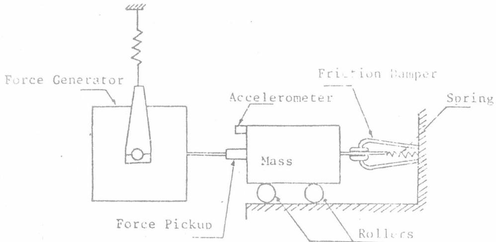
Fig.2 - Experimental arrangement for determination of friction damper characteristics.
