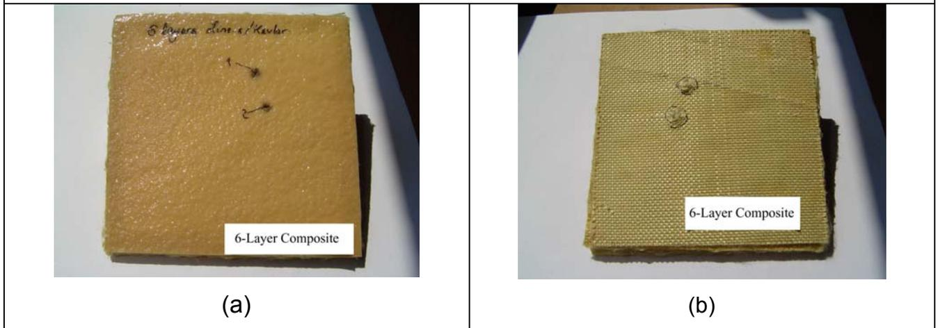
Fig. (30) A K/L-6 target perforated by 7.62 projectiles with different velocities at normal impact: (a) front face, and (b) back face
