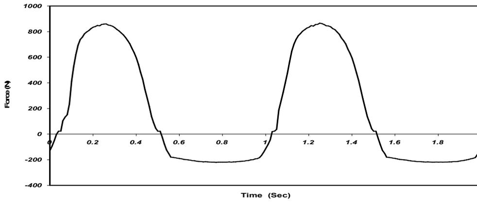
A- Force vs Time characteristics with input of frequency 1 Hz
