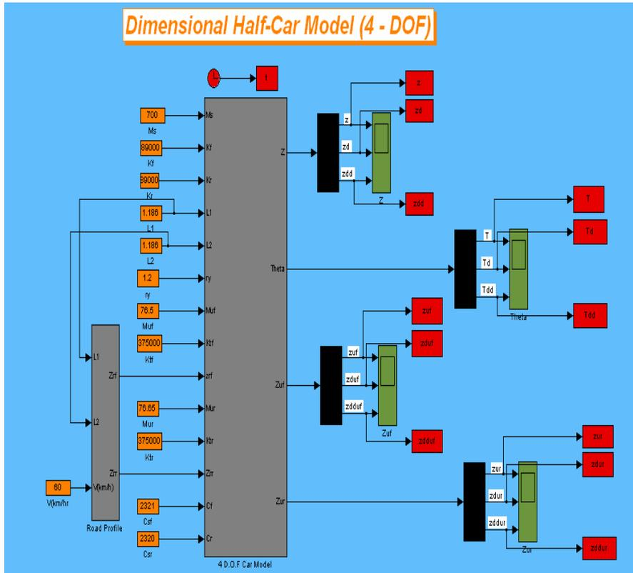
Fig. 2 (a) The half car model using Simulink
