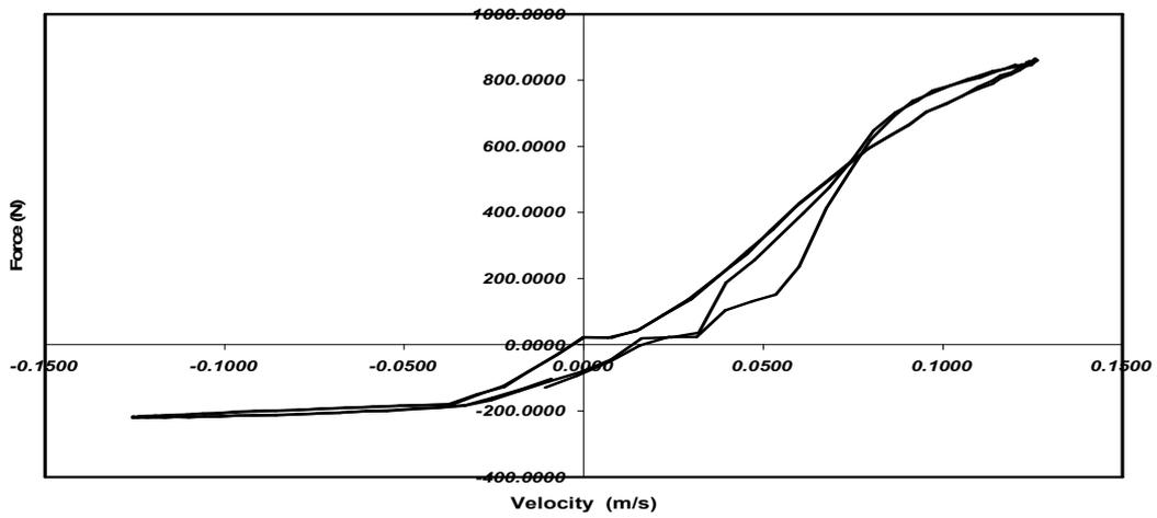
C- Force vs Velocity characteristics with input of frequency 1 Hz
