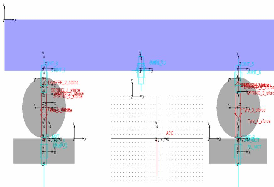
Fig. 2(b): Half car model using ADAMS
