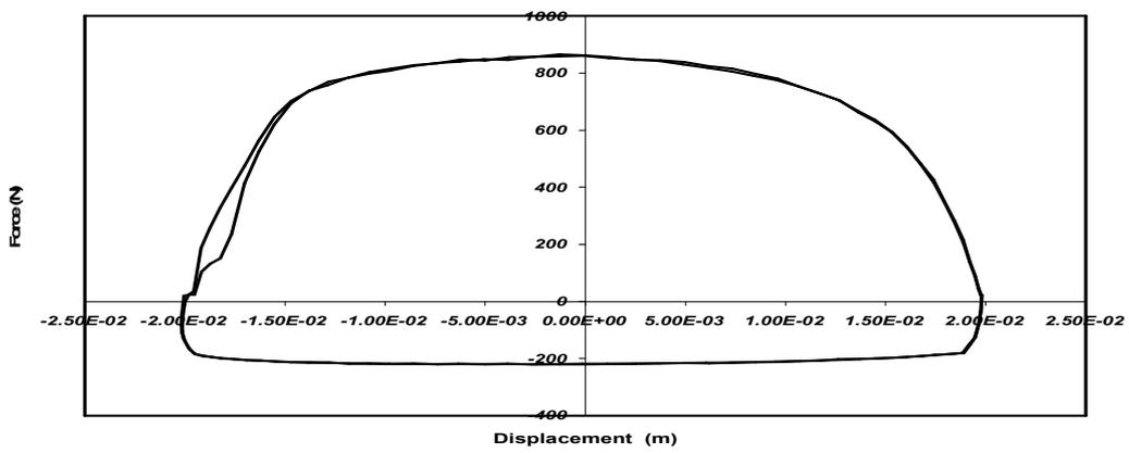
B- Force vs Displacement characteristics with input of frequency 1 Hz
