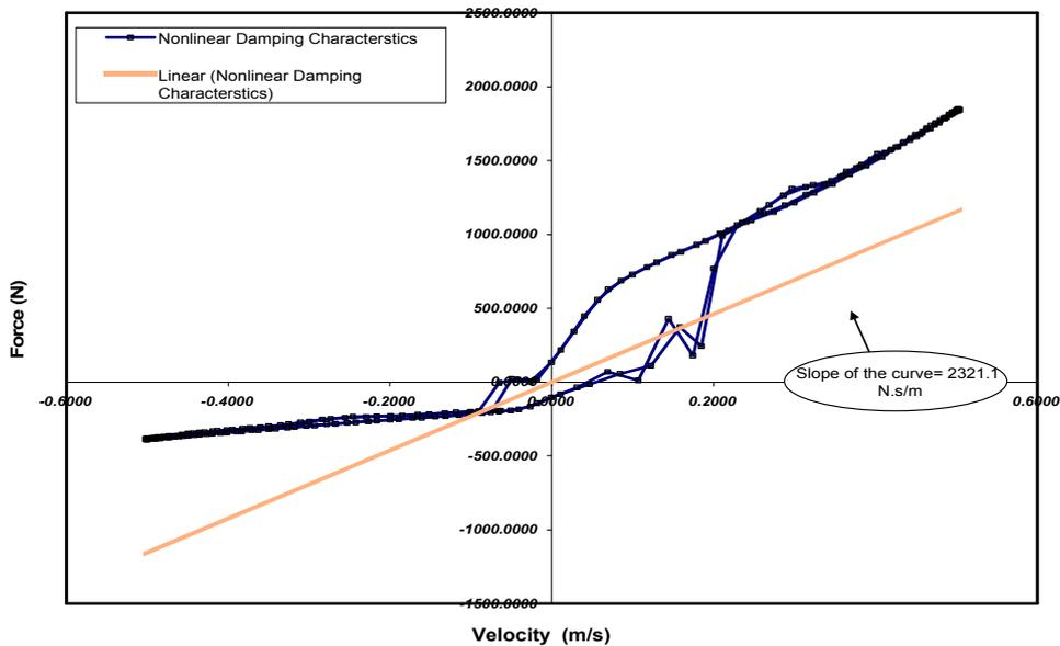
Fig. 6: Vehicle front linear damping approximation
