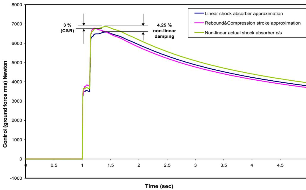
Fig. 10: Vehicle dynamic tire force (control)
