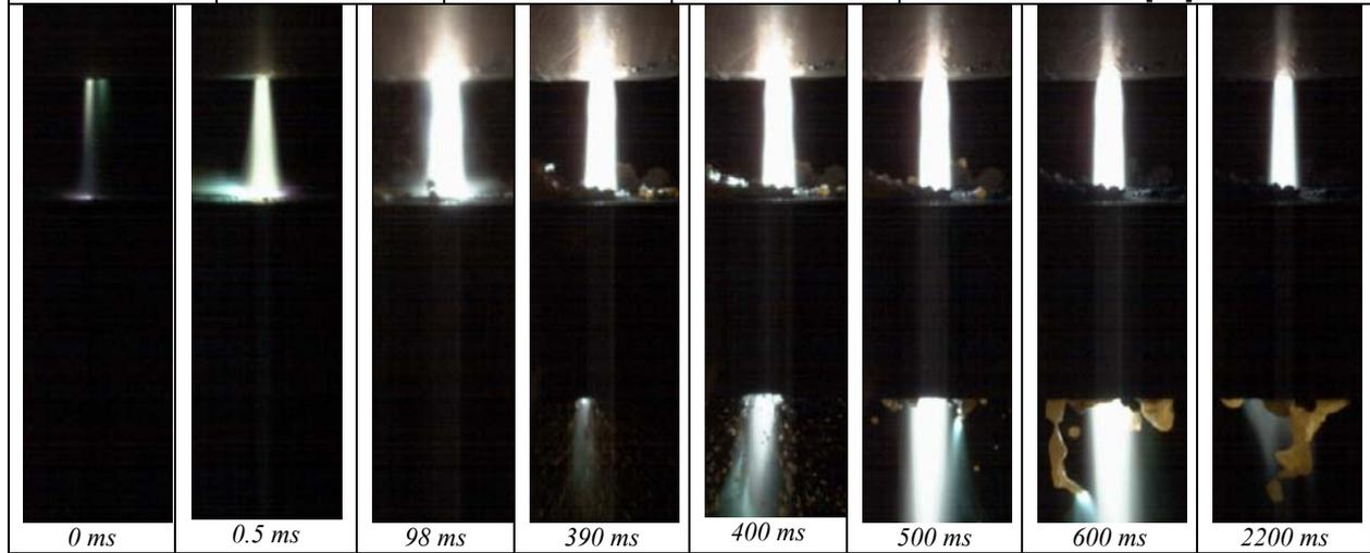
Figure 13. Piercing of a 15 mm SS slab (1.6 mm nozzle, 100 A, pilot arc plasma/shield gas:  $\text{N}_2/\text{N}_2$ , cut plasma/shield gas:  $\text{H35}/\text{N}_2$ , 1,000 fps, 1/20,000 shutter time). Multiple arc root attachments from plasma jet through conductive metal vapour projecting from dross nodules accumulated around the pierce bottom edge can also be seen in frames from 400 to 600 ms. Pictures taken from [20]
