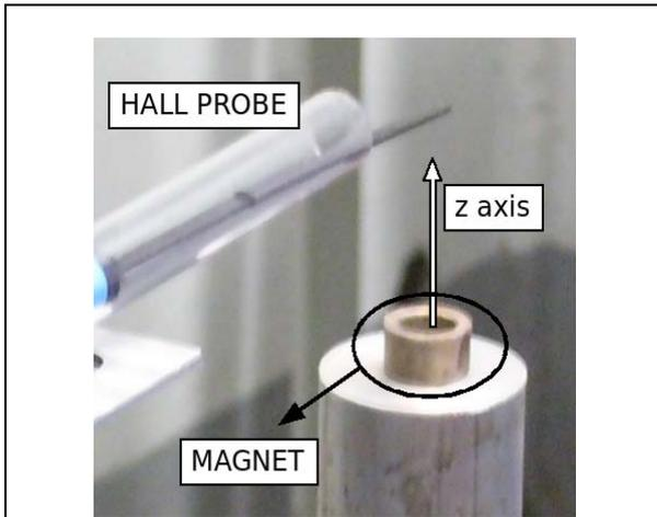
Fig. 7. Experimental setup for 2-D reconstruction with Hall effect probe of magnetic flux generated by the permanent magnet embedded in the Komatsu torch (internal diameter: 10mm; external diameter: 14.8mm; height: 8mm) as from patent [12]. Picture taken from [22].
