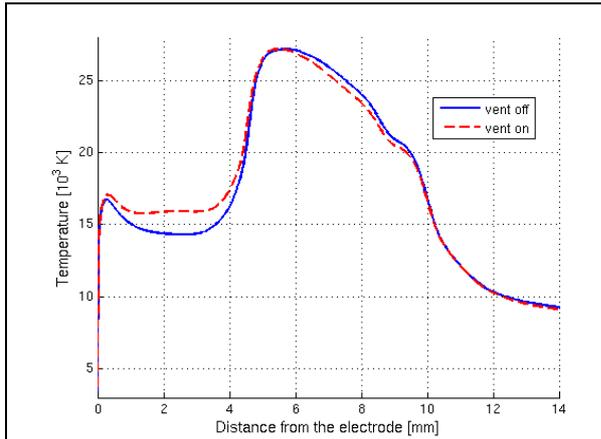
Fig. 1. Plasma temperature [K] on the torch axis from simulation for the vented and non-vented case. Picture taken from [22].
