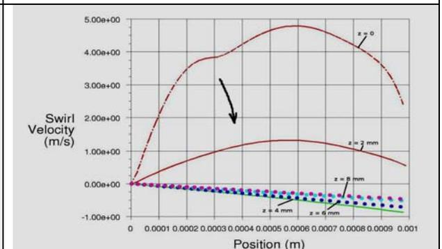
Fig. 6. Plasma swirl velocity at a distance  $z$  [mm] downstream torch shield along the radius of the jet with anticlockwise swirl of the secondary gas. Picture taken from [22].
