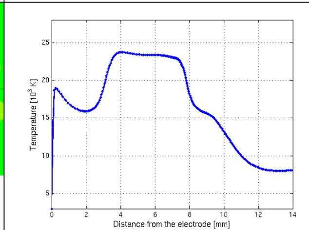
Fig. 10. Plasma temperature [K] on the axis of the torch from simulation for the Komatsu plasma torch with magnetization apparatus under operating conditions as in Fig. 9. Picture taken from [22].
