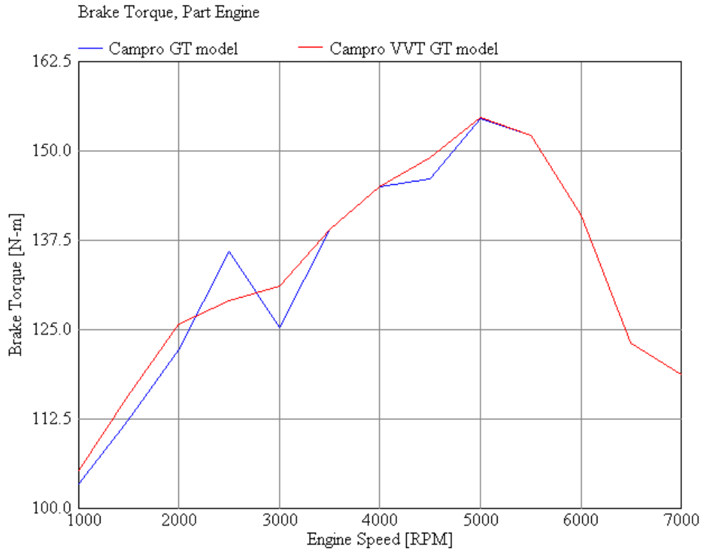
Fig. 15 Comparison of torque for CAMPRO GT model and CAMPRO GT model equipped with the Variable Valve Timing system
