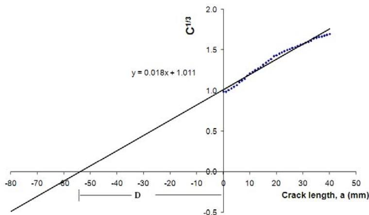
Fig. 6. Graph of  $C^{1/3}$  versus crack length ( $a$ ) for corrected beam theory
