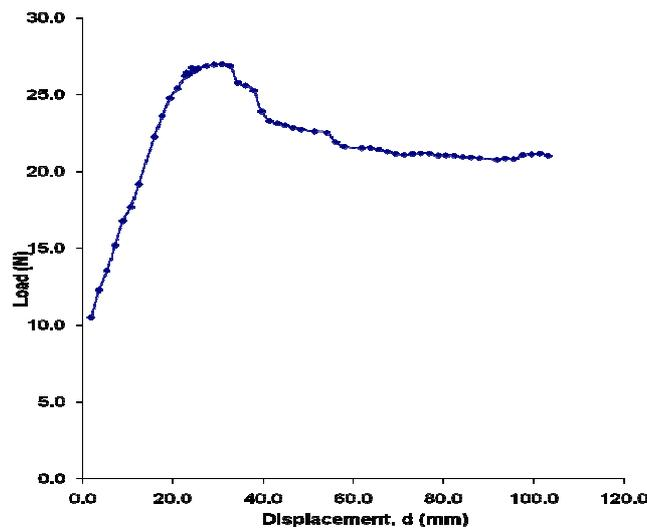
Fig. 5. Graph of load ( $P$ ) against displacement ( $d$ ) for 10 layers silk fibre
