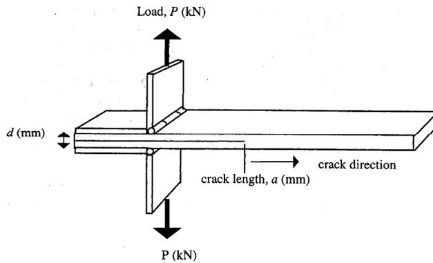
Fig. 2. Geometry of the double cantilever beam specimen
