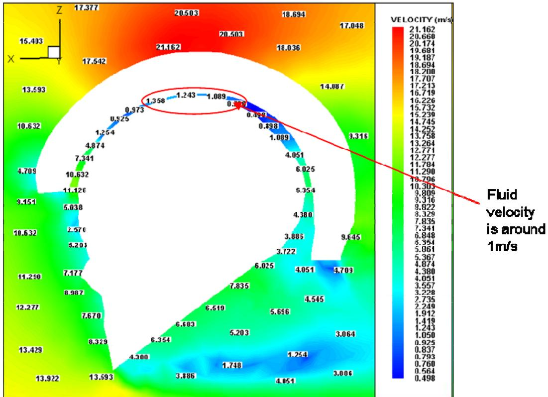
Fig 2: Velocity Contour values on the central x-z plane within and outside the gap of a helmet without ventilation.
