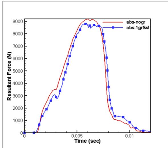
Fig 7: Total force on the head with and without ventilation in helmet
