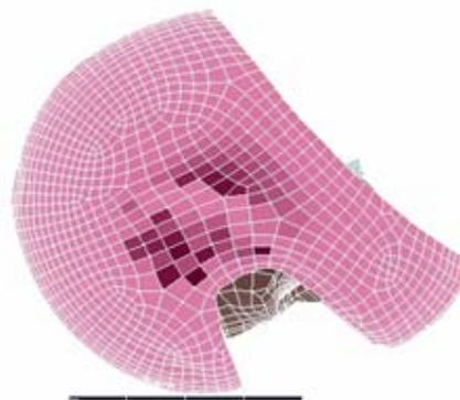
Fig 5: Finite element model of helmet-head in front impact
