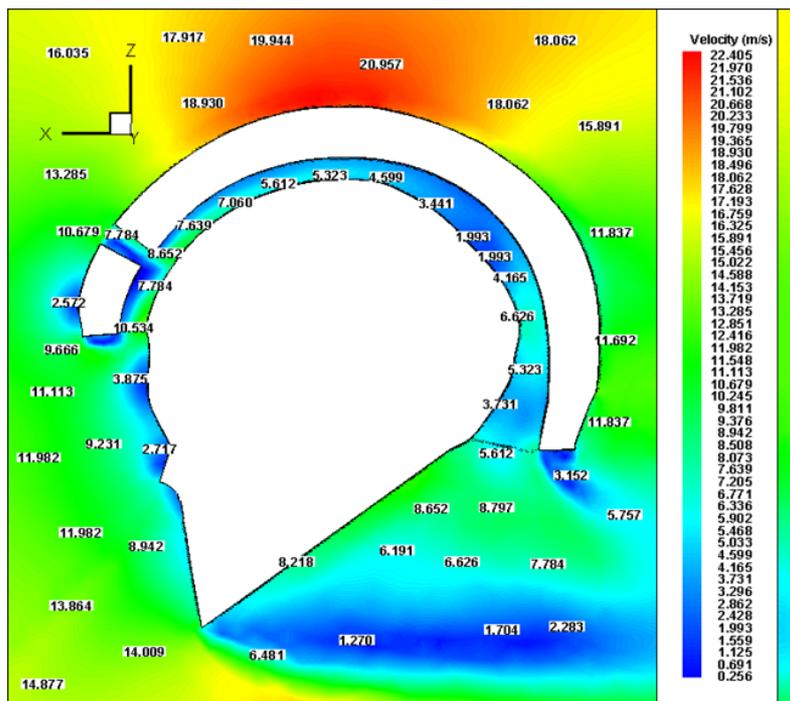
Fig 4: Velocity contour values on the central x-z plane in and outside the gap with 14mm x 7mm groove and 48mm x 7mm slot
