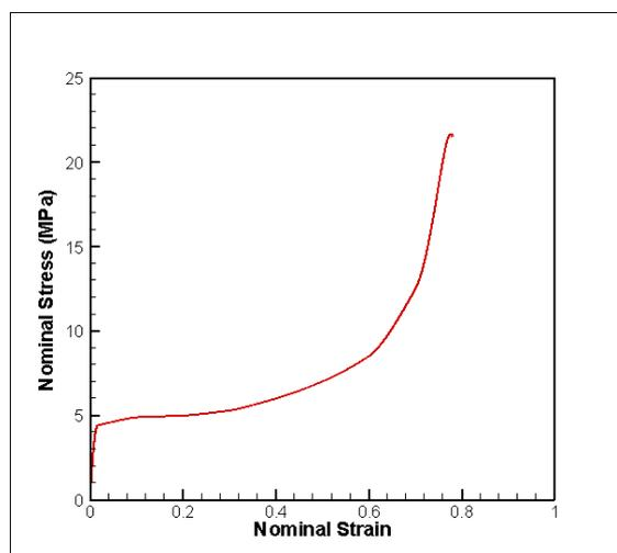
Fig 6: Stress-strain relation for Aluminum foam of 300 kg.m<sup>-3</sup> density
