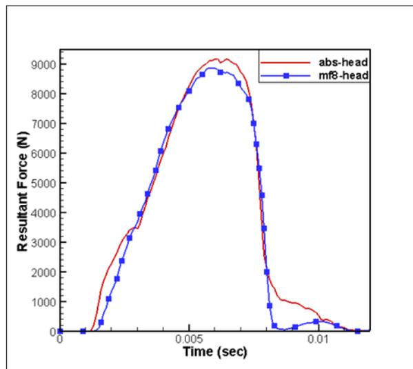
Fig 8: Total force on the head with helmets of ABS shell and Metal foam shell
