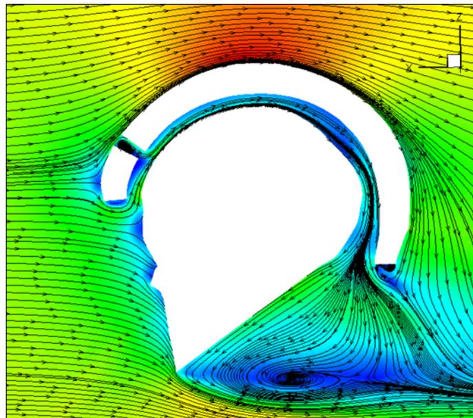
Fig 3: Streamlines in and outside the gap on the central x-z plane in helmet with 14mm x 7mm groove and 48mm x 7mm slot.
