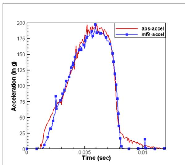
Fig 9: Acceleration in 'g' of the head with helmets of ABS shell and Metal foam shell
