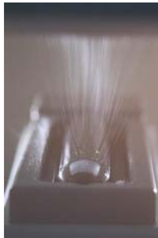
Fig. 3. Rotating roller, immersed in a polymer solution
