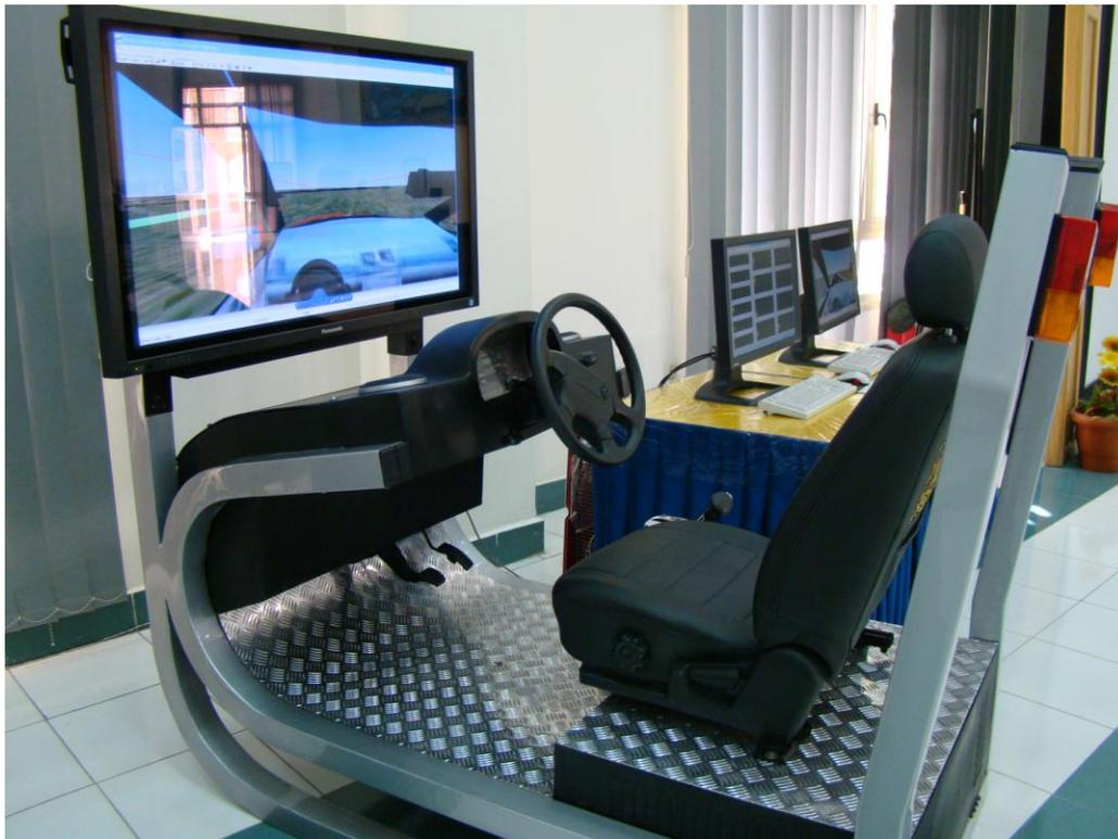
**Figure (4)** *The Driving Simulator Developed at the Military Technical College*
