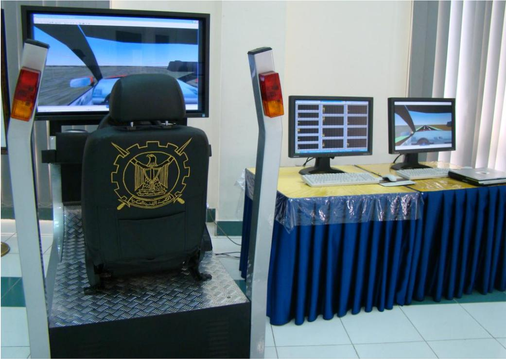
Figure (5) The Driving Simulator Developed at the Military Technical College
