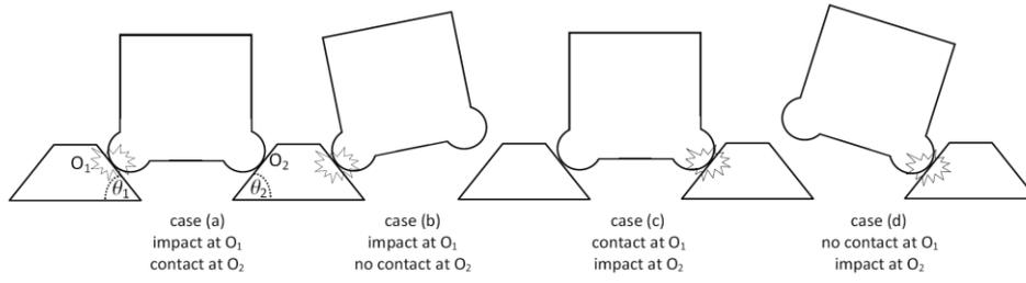
**Figure (3): Rigid block contact-impact cases**
