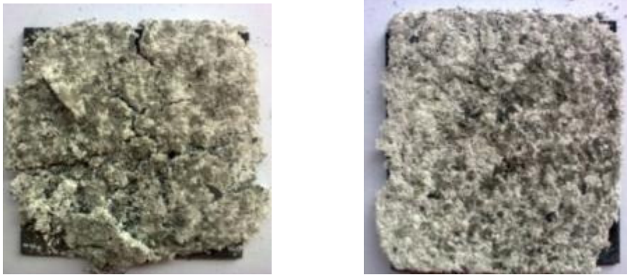
Fig. 3. After fire test at 850 °C.
