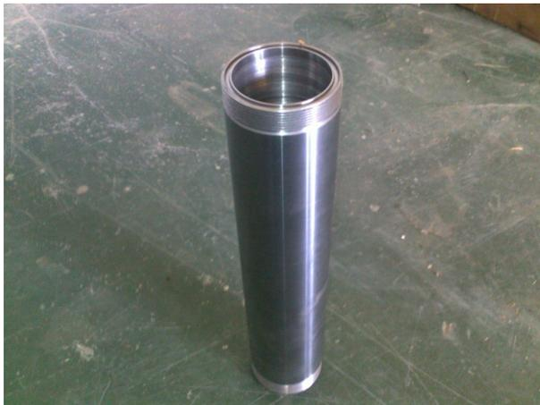
**Fig. 7.** Combustion chamber of modified two-inch motor.
