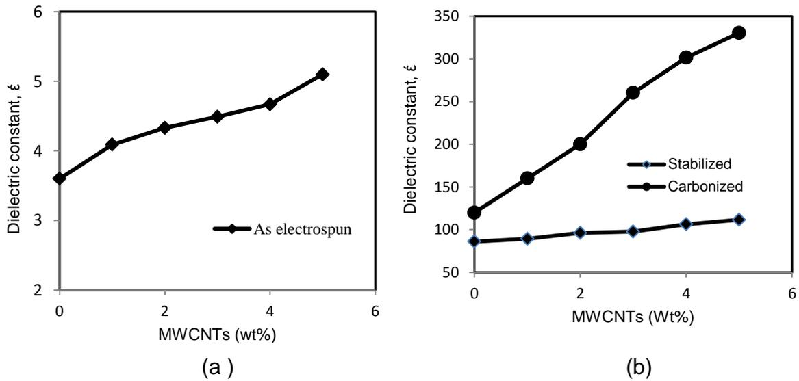
**Fig. 2.** (a) Dielectric constant as electrospun and (b) Dielectric constant satablization and carbonization for avs. MWCNTs (Wt %) at frequency 25000 Hz.
