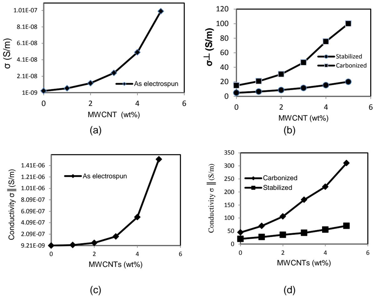
**Fig.4.** Electrical conductivity of nanofiber fabric as a function of MWCNT concentration in terms of heat treatment (a) vertical component as electrospinning; (b) vertical component at stabilization and carbonization; (c) parallel direction As electrospun and (d) parallel component at stabilization and carbonization.
