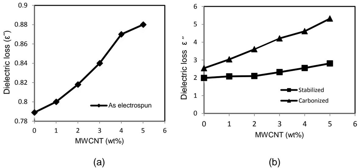
**Fig. 3.** (a) Dielectric loss PAN nanofiber as electrospun and (b) stabilization and carbonization PAN nanofiber for avgs. MWCNTs (wt %) at frequency 25000 Hz.
