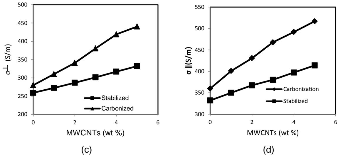
**Fig.5.** Electrical conductivity of MWCNTs/carbon single nanofibril composites in terms of heat treatment (a) vertical component as electrospinning; (b) parallel direction As electrospun; (c) vertical component at stabilization and carbonization and (d) parallel component at stabilization and carbonization.
