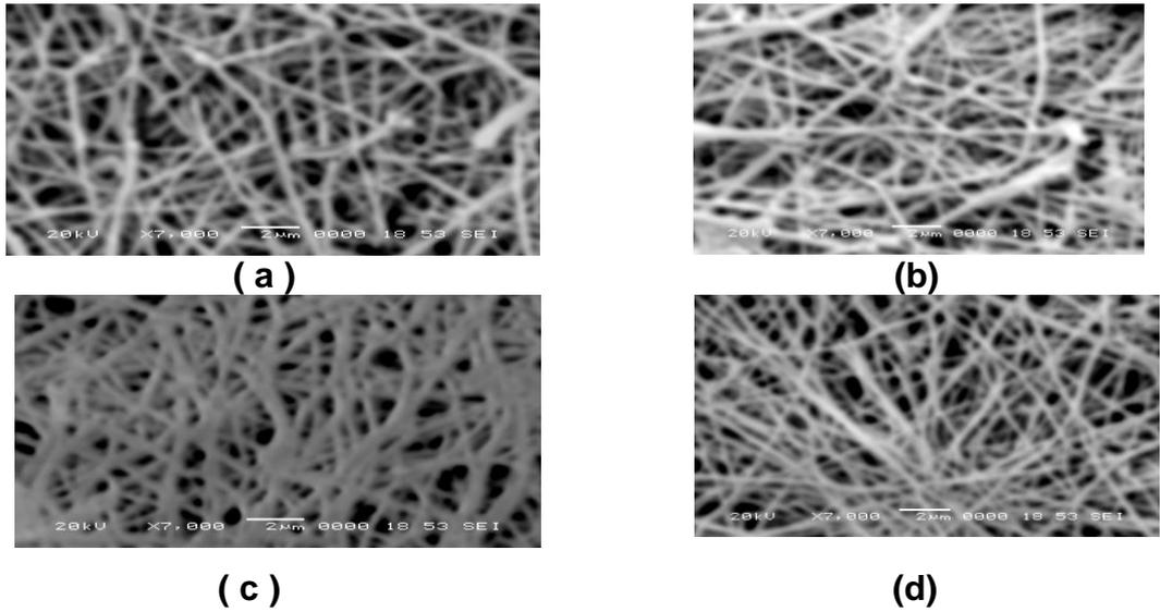
**Fig.1.** SEM micrographs of composites CNF: (a) Pure PAN As electrospun, (b) Pure PAN hot pressed, (c) 5% MWCNT in PAN As electrospun, (d) 5% MWCNT in PAN hot pressed.
