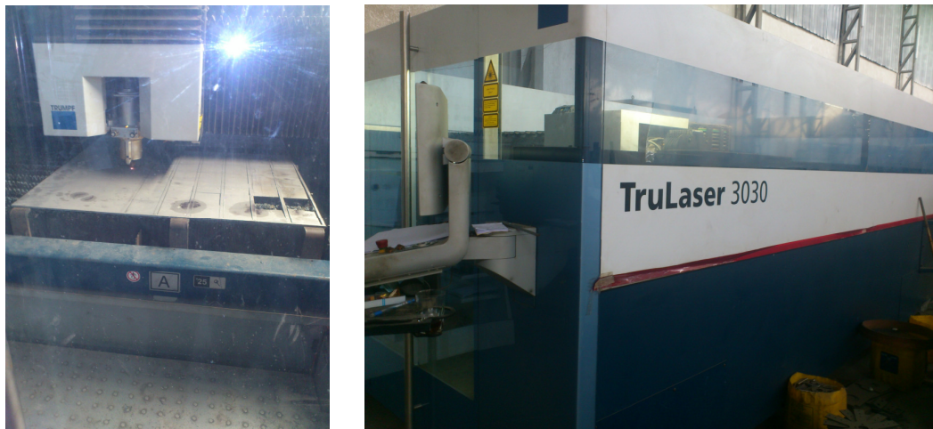
Fig. 1. The Laser Machine type (TruLaser 3030) used in cutting plates and test specimens.
