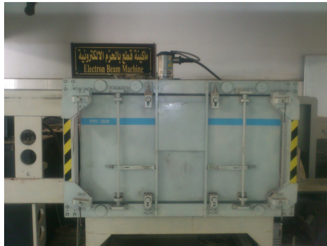
Fig. 2. The Chamber of the used Electron Beam Welding Machine.
