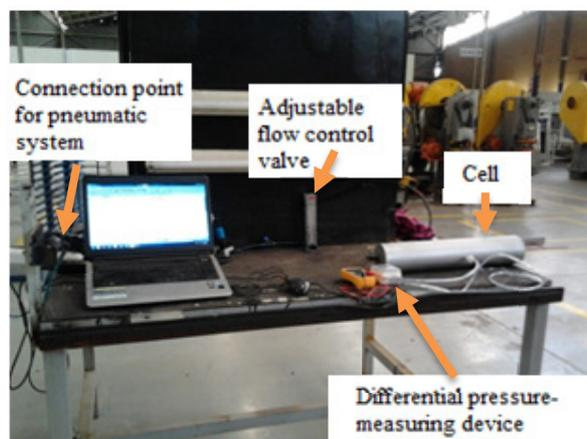
**Fig.5.** Airflow resistivity test setup.
