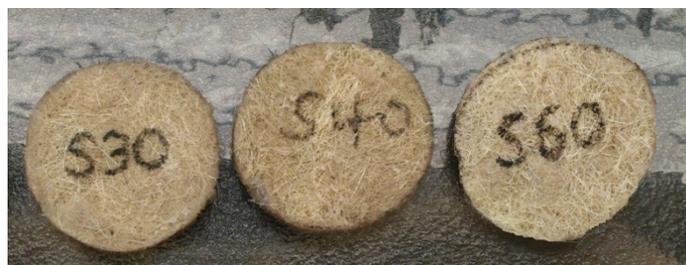
**Fig.4.** Kenaf/sisal natural fibre circular specimens.
