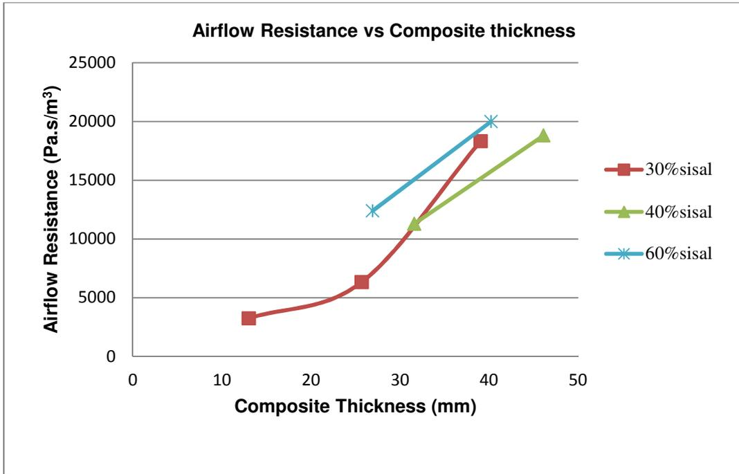
**Fig.6.** Airflow resistance verse composite thickness.
