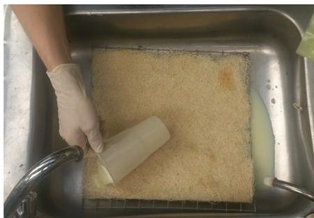
**Fig.3.** Coating natural fibres with ABS.
