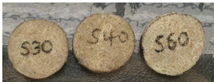
**Fig.4.** Kenaf/sisal natural fibre circular specimens.
