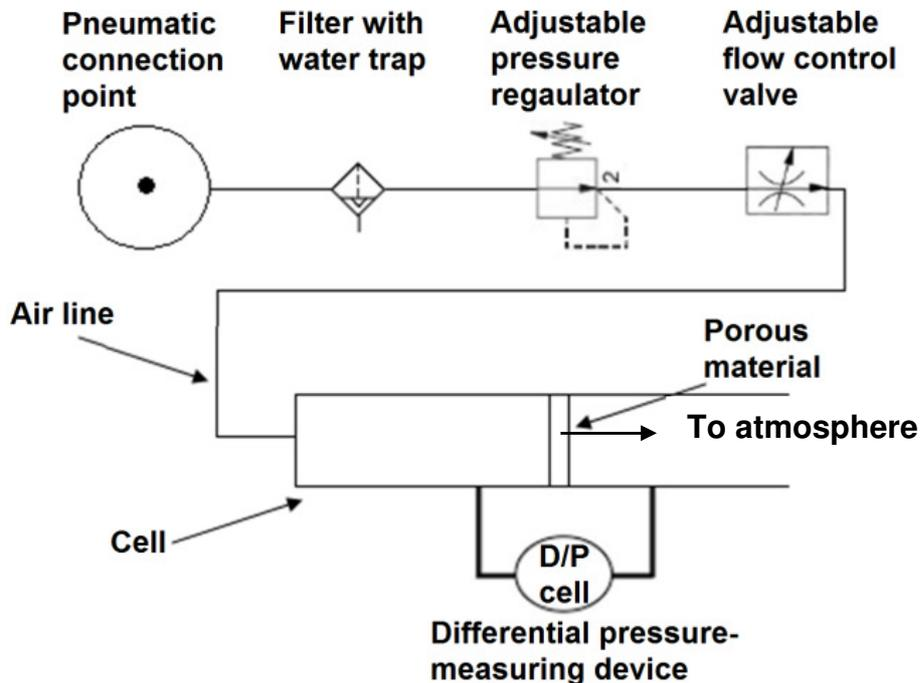
**Fig.1.** Schematic setup of airflow resistivity test.
