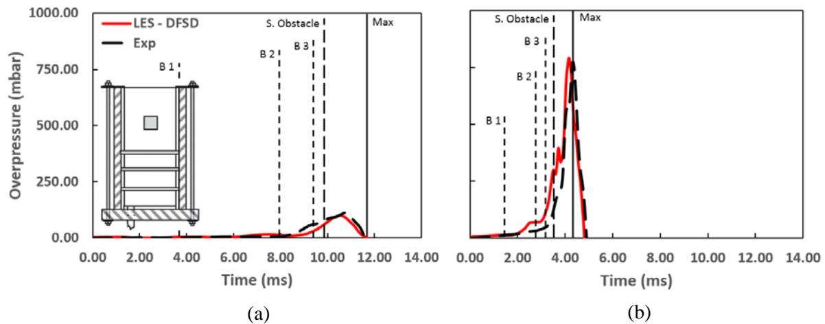
**Figure 6.** Overpressure-time traces for propane-air at  $\Phi=1.0$  (a) hydrogen-air at  $\Phi=0.7$  (b) using configuration BBBS.
