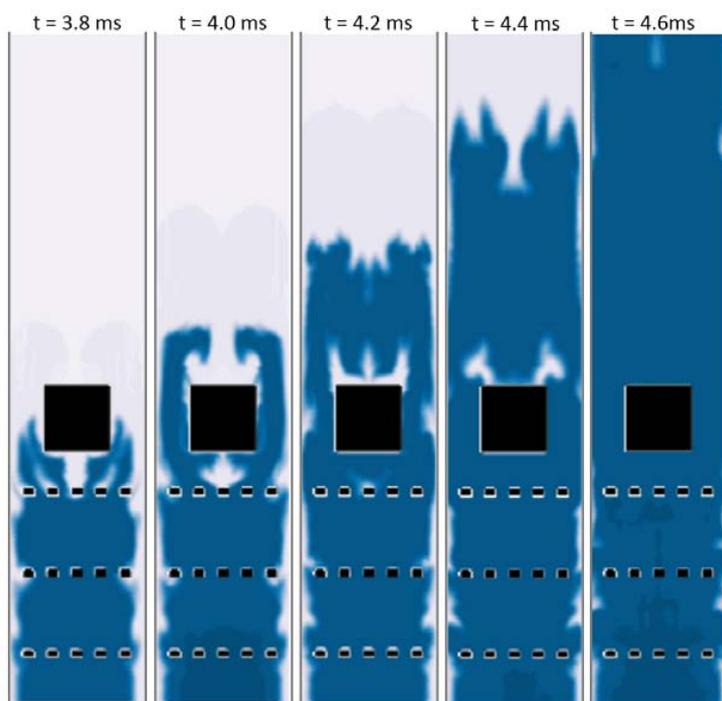
**Figure 5.** Numerical results showing Iso-lines of the reaction progress variable on the chamber midplane for hydrogen-air flames.
