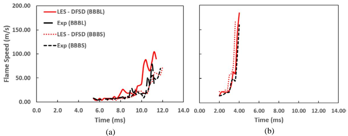
**Figure 8.** Speed-time traces for propane-air at  $\Phi=1.0$  (a) hydrogen-air at  $\Phi=0.7$  (b).
