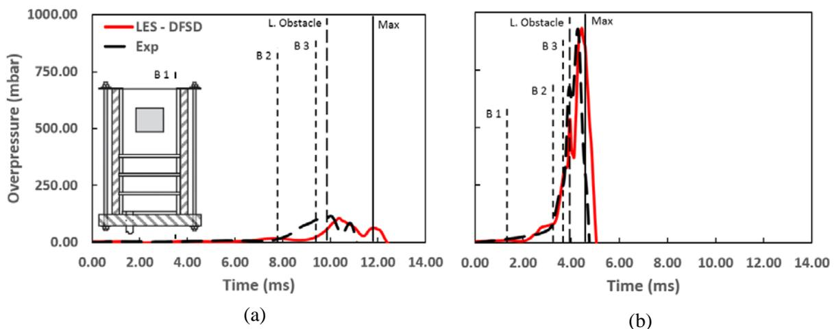
**Figure 7.** Overpressure-time traces for propane-air at  $\Phi=1.0$  (a) hydrogen-air at  $\Phi=0.7$  (b) using configuration BBBL.
