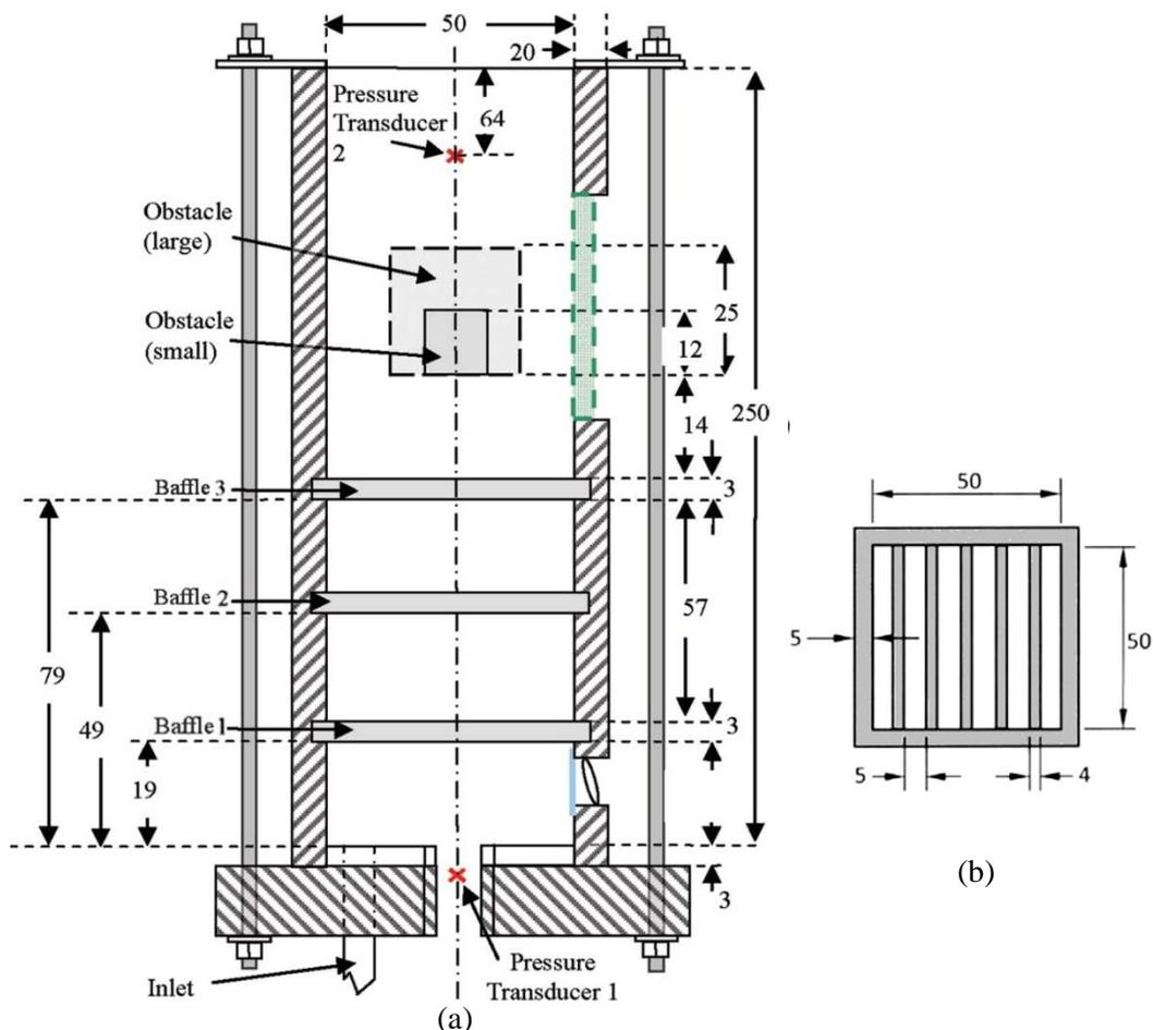
**Figure 1.** Chamber schematic (a) and removable baffle (b) (all dimensions in mm, not to scale).
