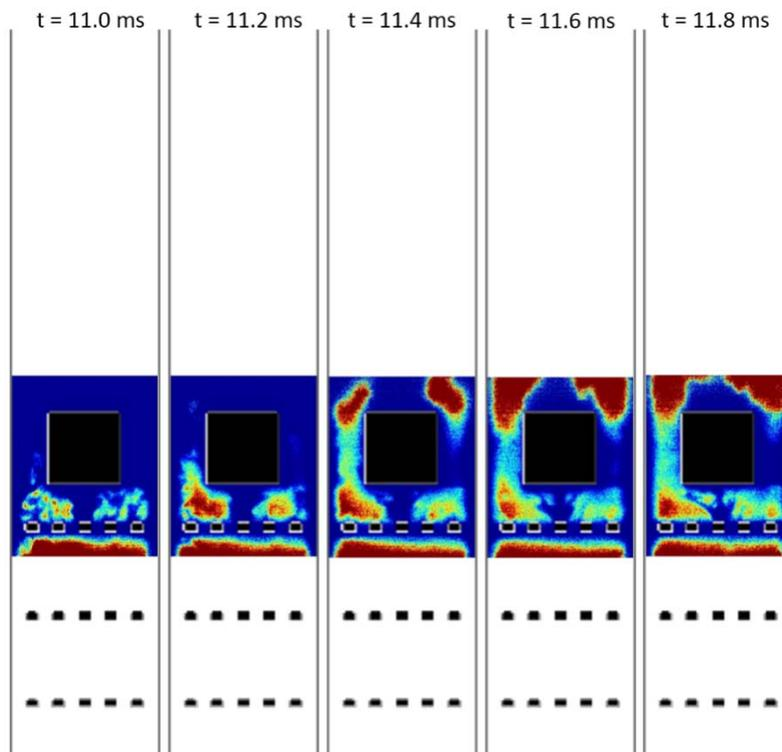
**Figure 3.** High Speed LIF-OH images of propane-air flame structure at different times after ignition.
