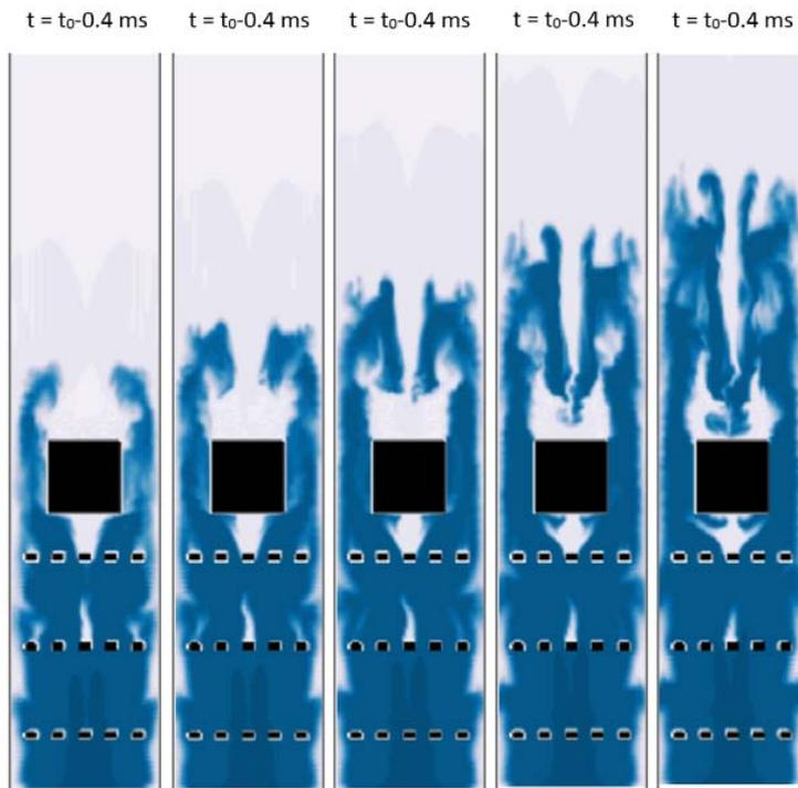
**Figure 4.** Numerical results showing Iso-lines of the reaction progress variable on the chamber midplane for propane-air flames.
