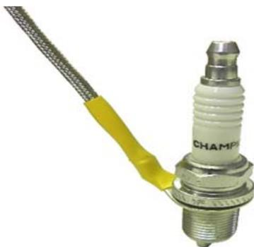
**Figure 9.a.** Spark plug temperature sensor installation.
