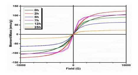
**Fig. 4.** Hysteresis curves of mechanically alloyed Fe-50wt.% Cu powder with different times.
