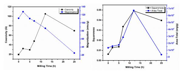
**Fig. 5.** Milling Time dependence of mechanically alloyed Fe-50wt.% Cu powder; (a) Coercivity and magnetization and (b) Squareness and Area-Total.
