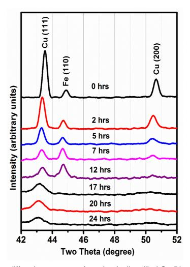
**Fig. 1.** X-ray diffraction patterns of mechanically milled Cu-50wt.%Fe powder at different milling time.
