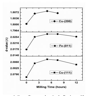
Fig. 2. D-values variation after mechanical alloying with different time.
